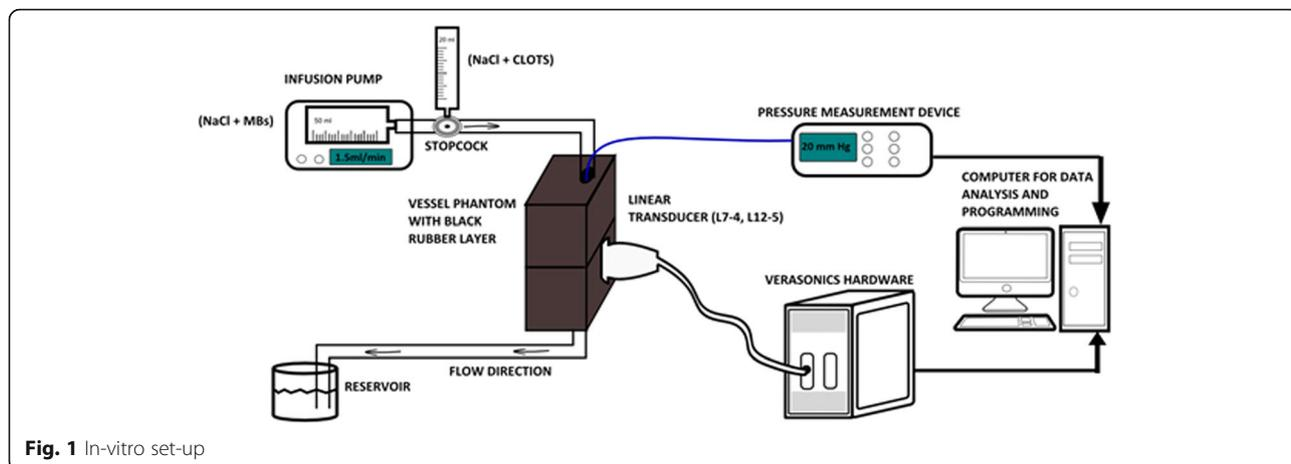
**Fig. 1** In-vitro set-up
